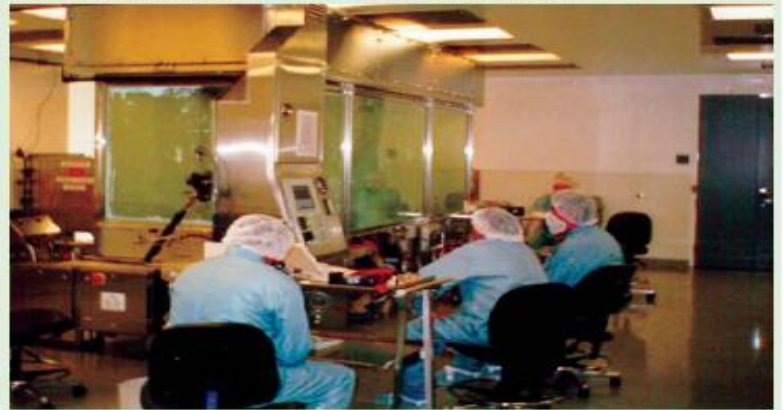
Photo 1: Aseptic fill isolator undergoing chlorine dioxide disinfection
