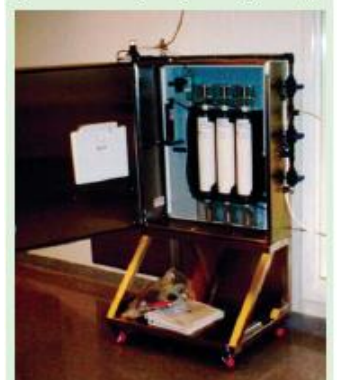
Photo 2: Prototype chlorine dioxide gas generator showing CD-generating cartridges
