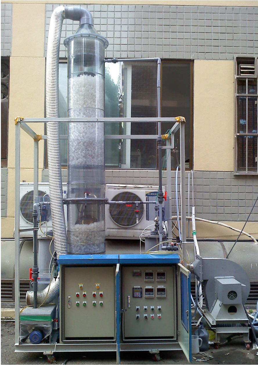
Figure 3.4 Photograph of the wet scrubber
